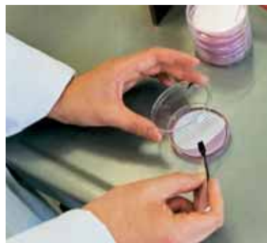
Place the filter on the pad without entrapping air bubbles
