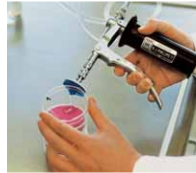
Wet the nutrient pads with 3.5 ml sterile and distilled or demineralized water
