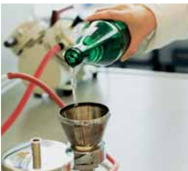
Filter the sample. Then rinse the inside of the filter holder with sterile water or physiological saline solution
