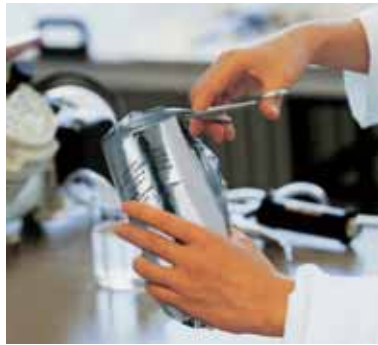
Cut open the packaging and remove the number of nutrient pads needed
