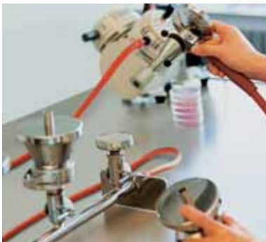
Open the vacuum tap. Flame the frit and close the vacuum tap
