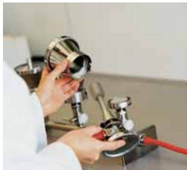
Flame the stainless steel funnel
