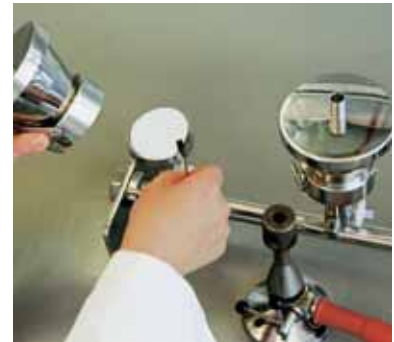
Place the filter on the frit of the filter holder. In case of a yellow protective disc make sure to discard it before assembling the funnel or the top part of the filter holder.
