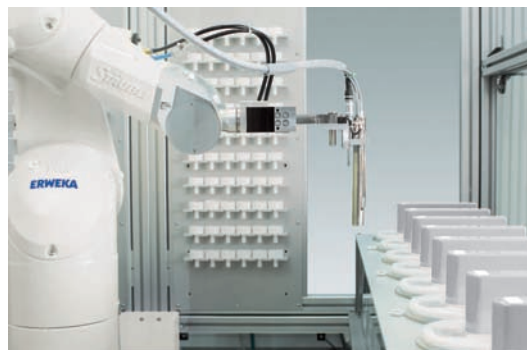
Robot arm with UV-optrode (Fibre Optics) taking measurement inside the vessel
