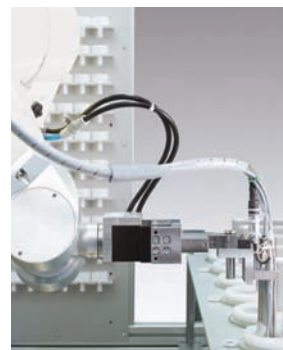
Robot arm with UV-optrode (Fibre Optics) taking measurement inside the vessel
