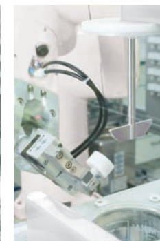
Insertion of sample with Japanese sinker/Removal of Japanese sinker
