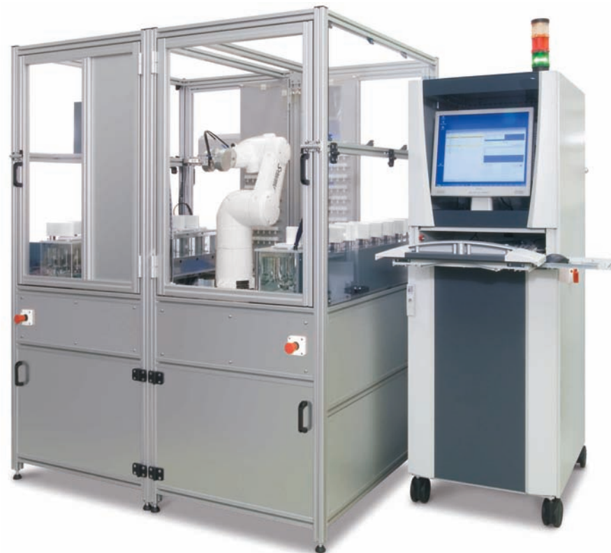
Robot arm with UV-optrode (Fibre Optics) taking measurement inside the vessel
